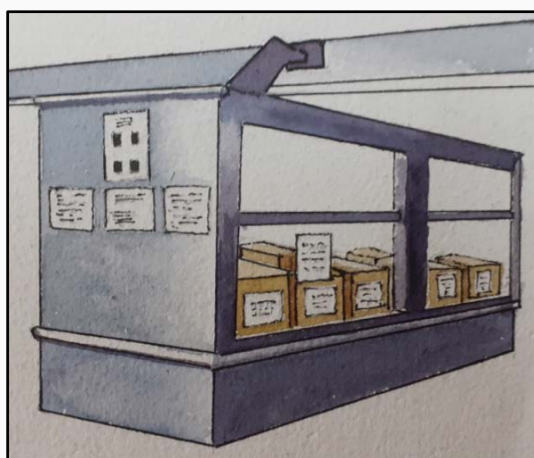
Figure 12: Fuming hood ventilation for dye storage
