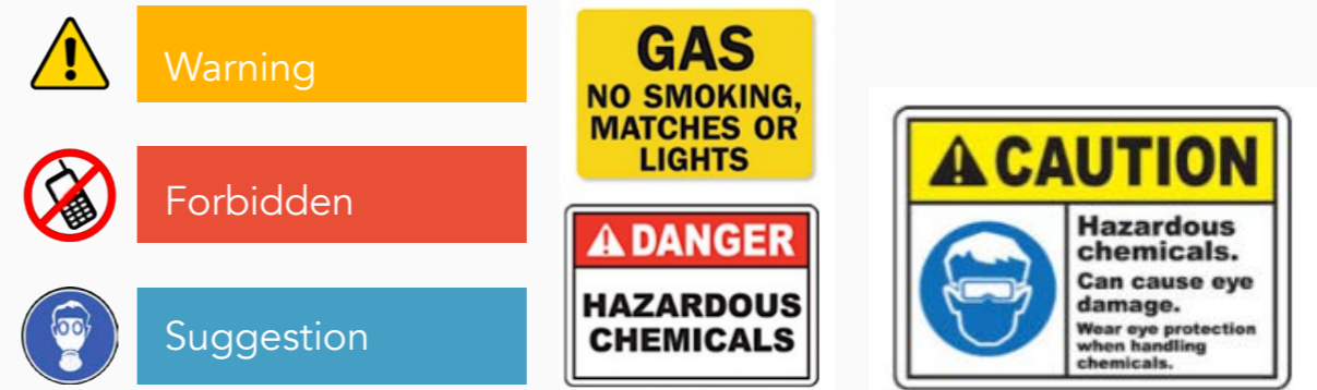
Figure 09: Examples of signages to communicate hazards at critical places in a facility
