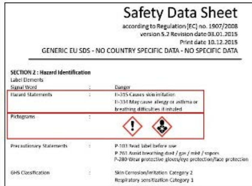
Figure 06: Example of a hazard identification from a section 2 of a Safety Data Sheet (SDS)
