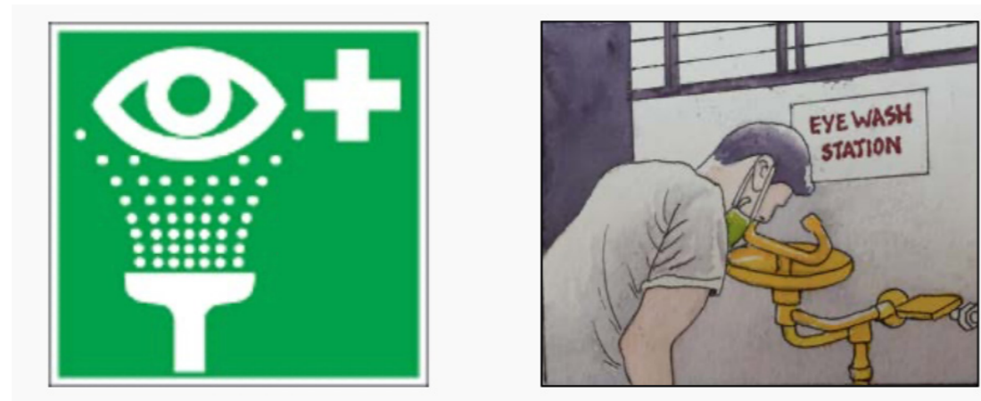
Figure 9: Signage for eye wash station and eyewash stand
