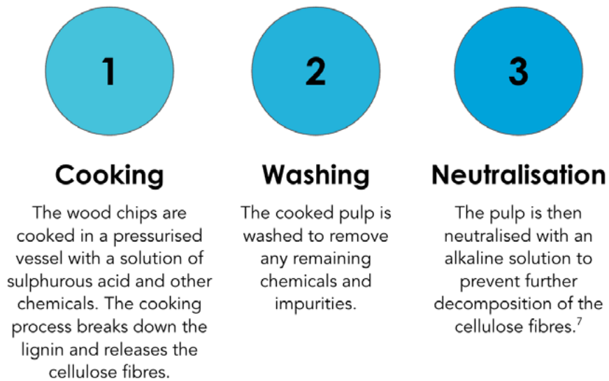
Figure 3: Key Steps in the Sulphite Pulping Process
