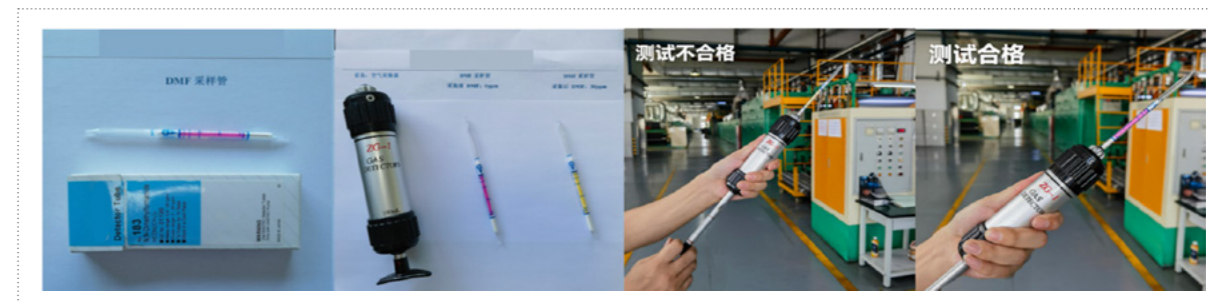
Figure 8: Handheld DMFa detection system (Photo courtesy Lishui Heli New Material, Lishui, China)
