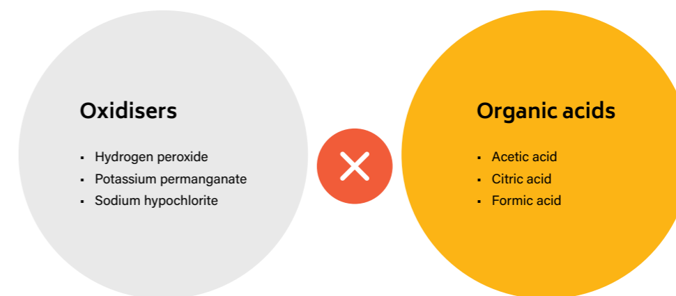
Figure 5: Oxidisers should not be stored with organic acids
